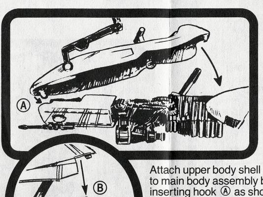
Attach upper body shell to main body assembly by inserting hook (a) as shown and press upper body shell down firmly until it snaps into place on the main body assembly (B).
